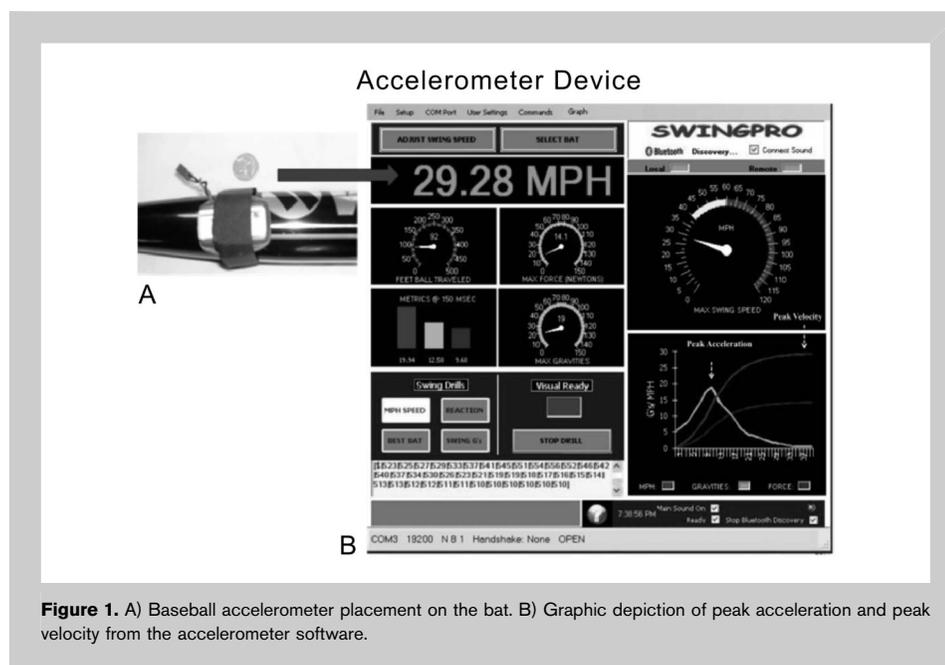
**Figure 1.** A) Baseball accelerometer placement on the bat. B) Graphic depiction of peak acceleration and peak velocity from the accelerometer software.
