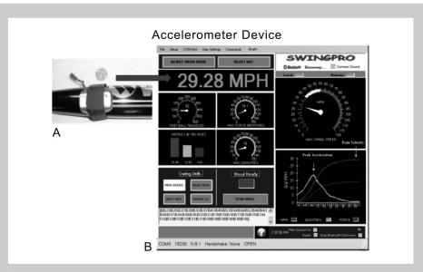
Figure 1. A) Baseball accelerometer placement on the bat. B) Graphic depiction of peak acceleration and peak velocity from the accelerometer software.
